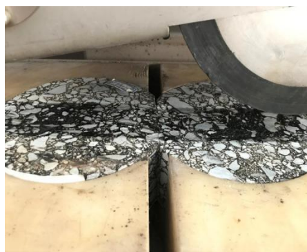
Fig. 3 Core specimen in test
