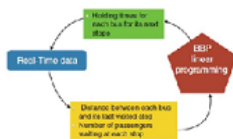
Fig. 3 Framework for interleaving optimization (BBP LP modeling) and real time data retrieving (or simulation). Source Hernández Landa et. al (2015)
