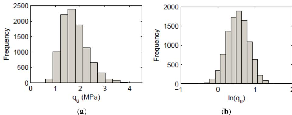
**Figure 3.** Histograms of resultant strength calculated with Eq. 3 from the data shown in **Figure 2**. (a) Unconfined compressive strength  $q_u$ , (b)  $\ln(q_u)$
