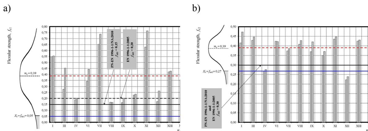
Figure 6. Tests results: a) flexural strength  $f_{x1}$ , b) flexural strength  $f_{x2}$
