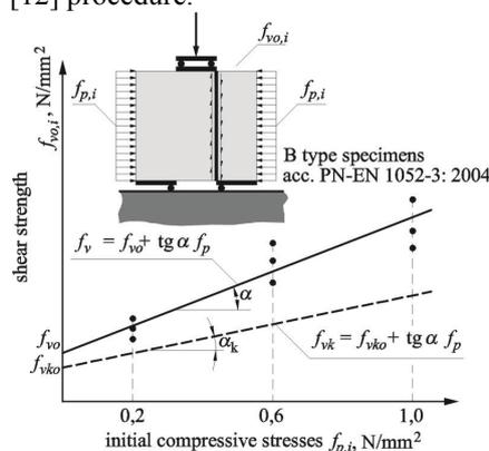
**Figure 1.** The shape of the specimens and the basic symbol
