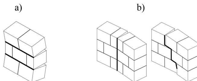
**Figure 4.** Flexural failure of masonry in plane: a) parallel, b) perpendicular to the bed joints
