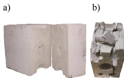
**Figure 3.** Failure patterns units at  $f_p = 1,0 \text{ N/mm}^2$ : a) units II series, b) units XIV series
