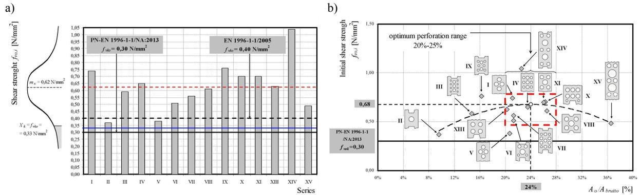
**Figure 2.** Test results of  $f_{vko}$ : a) a comparison with the values prescribed by the EN 1996-1-1: 2005 and EN 1996-1-1: 2013, b) as a function of the percentage area of openings
