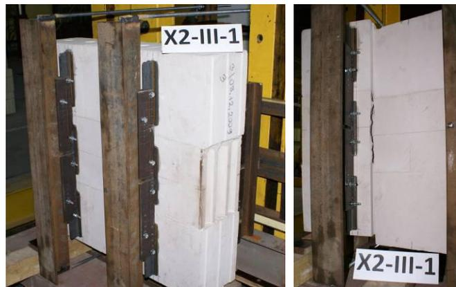
Figure 5. Flexural strength test
