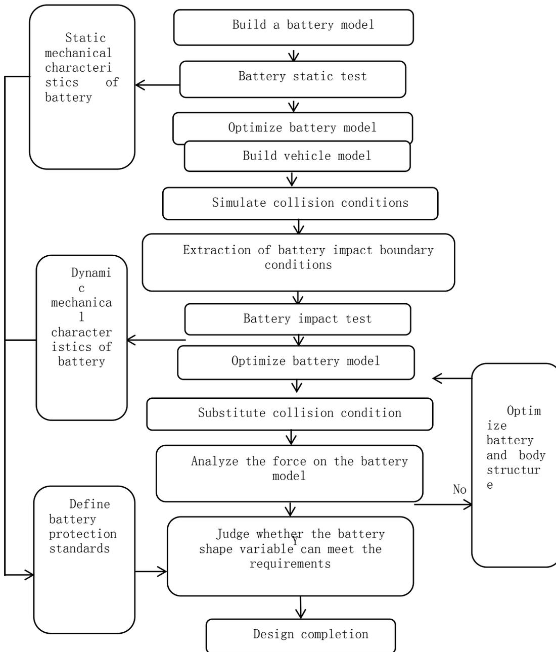
Figure 2 New Battery Collision Safety Design Process
